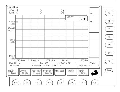
(5) Set the Span (sweep width) to 50 nm.
