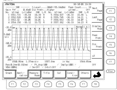
In the SNR mode, the wavelength, level, and SNR of up to 8 peaks can be displayed simultaneously.
