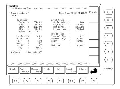
Input the number in the range 1 to 5 at Memory Number at the top left of the screen using the Data entry keys. The current settings are saved when the Execute function key (f1) is pressed.
