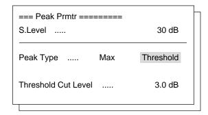
Set the target for peaks to be analyzed up to X dB below the maximum peak at S.Level in the Peak Prmtr window. Select whether to use the wavelength of the point with the maximum measured level (MAX), or the center wavelength using Threshold analysis (Threshold) as the peak wavelength detection method at Peak Type. In both cases, the peak level is the level of the point measured as the peak.
