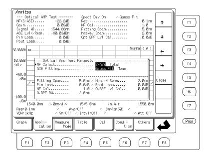
The following function keys are displayed in the Functions display field at right-hand side of the screen. Use the function keys to select the item indicated by the reverse displayed cursor, and set the value using the Data entry keys or Knob.
