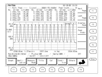
There are three display modes for WDM signal analysis: Multipeak, SNR, and Relative. (When Option 10 is installed, the Table display mode is added to these three modes.) The items displayed for each mode are different.
