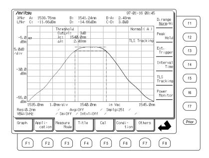
Note that during tracking measurement, the Auto measurement and the W1 Offset function key (f1) of the Cal card selected by pressing (F5) key is not passible to be used.
