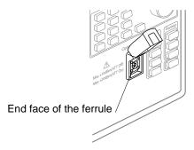
(4) Carefully refit the optical input connector taking care not to scratch or otherwise damage the end face of the ferrule.
