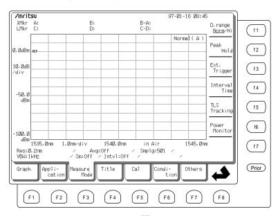
Press the Adjust to TLS function key (12) then select Execute by pressing the function key (11), which sets the measurement conditions automatically and start calibration. Calibration of the tracking wavelength will take about a few minutes.
