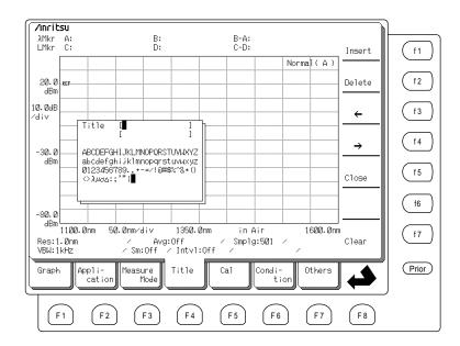
When the Title card is selected by pressing the F4 key, the character selection window shown above is displayed. Use the Knob to move the cursor to the position of the desired character, or use the function keys to move the cursor and insert a blank space. The following function keys are displayed in the Functions display field at right-hand side of the screen.
